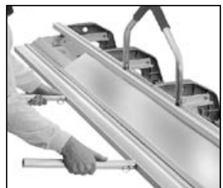
6 Lift the Bending Handles and compress the bend for a completed hem.
